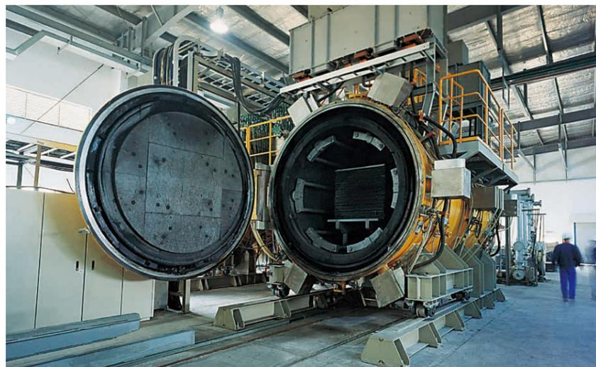
Large Sintering Furnace for Carbon-fiber Insulation (Kureha (Shanghai) Carbon Fiber Materials Co., Ltd.)
