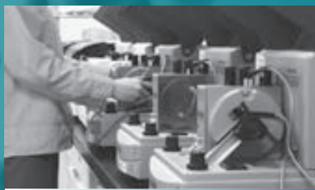
Measuring the oxygen permeability of films
