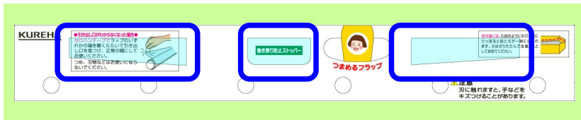
Embossed adhesive area to prevent the roll back of the film
