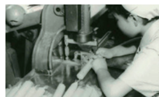
Sausage ligature process using a stamping machine
