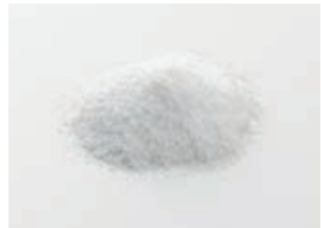
KF Polymer (polyvinylidene fluoride) binds electrodes in lithium-ion batteries
