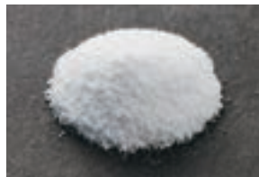
KF Polymer (polyvinylidene fluoride) binds electrodes in lithium-ion batteries
