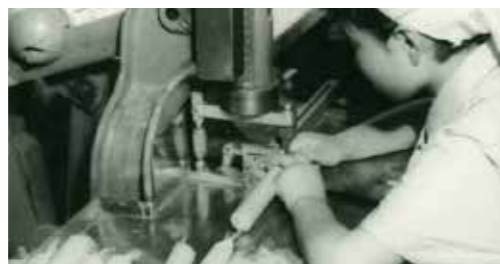
Sausage ligation process using a stamping machine
