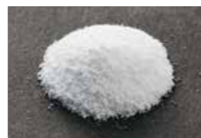
Polyvinylidene fluoride (PVDF) PVDF is a super engineering plastic with an excellent balance of chemical resistance and moldability, used in such fields as electronic materials and water treatment membranes.
